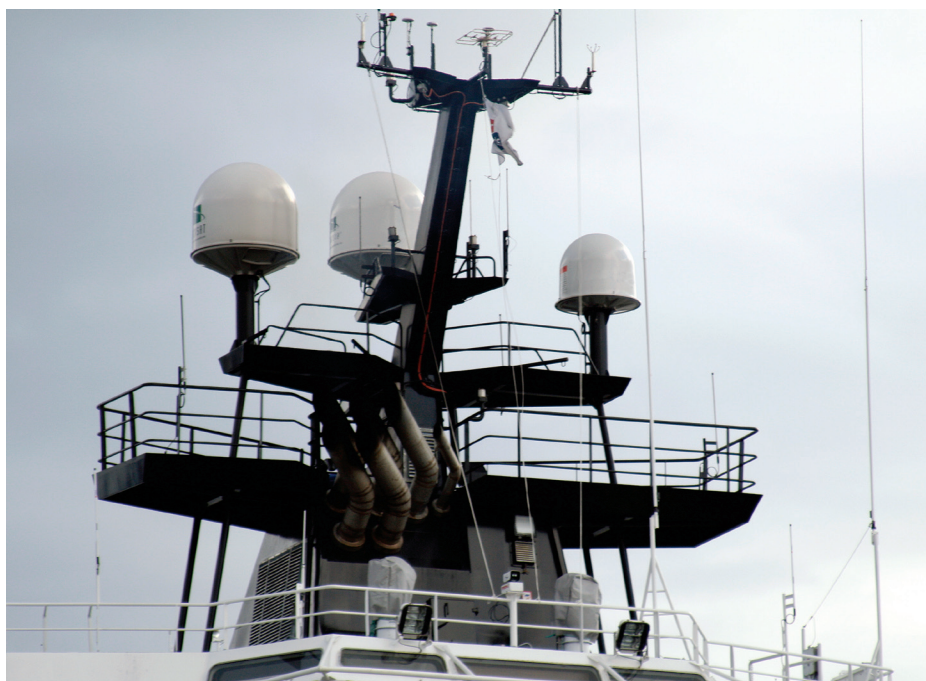
XpressLink provides both VSAT and FleetBroadband terminals, operating on two separate satellite networks [ photo: Stratos ]
