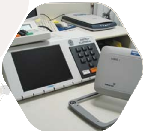
BGAN terminals like this one transmitted results gathered by electronic voting machines (left).
