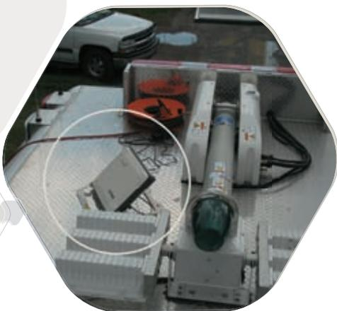
*Compact BGAN satellite terminal (circled) on top of a Hazmat vehicle, connected to a laptop, during a biological incident in rural Kentucky. Photo courtesy of Mark Garland, Murray State University.*
